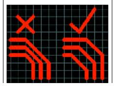
but through-linking will be harder. 65mil round or square pads for normal components and DIL ICs, with 0.8mm hole, will allow a 12.5 mil, down to 10 mil if you really need to. Centre-to-centre spacing of 12.5mil tracks should be 25 mil—slightly less may be possible if your printer can manage it. Take care to preserve the correct diagonal tracktrack spacing on mitered corners; grid is 25 mil and track width 12.5 mil.
