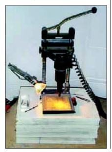
other and insert a 0.8mm track pin in two opposite corners, using the pins as pegs to line the PCBs up. Squeeze or hammer the pins into the boards, and then into the remaining holes. The two PCBs are now 'nailed' together accurately and can be drilled together.
